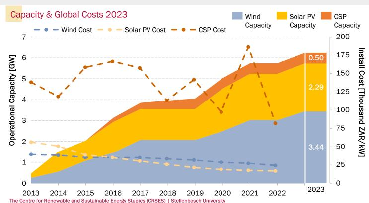
Renewable energy installed capacity and energy production are increasing in South Africa, but still constitute a small portion of the total capacity and energy mix. CSP costs are high and have more variability than wind and solar PV costs, which are both on a stable downward trend.
